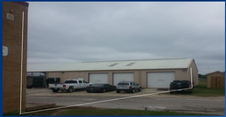
Maintenance drawing depicting a 2" underground conduit to provide a path for fiber run needed for connectivity
